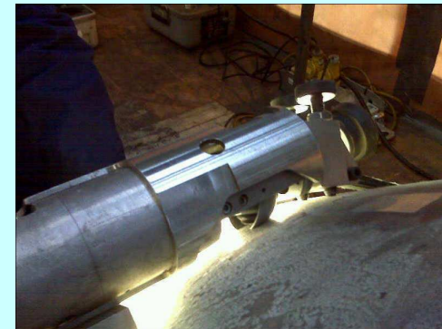
Scoop sampling in process on a pipework
